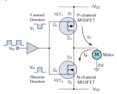
The two MOSFETs are configured to produce a bi-directional switch from a dual supply with the motor connected between the common drain connection and ground reference. When the input is LOW the P-channel MOSFET is switched-ON as its gate-source junction is negatively biased so the motor rotates in one direction. Only the positive +V<sub>DD</sub>supply rail is used to drive the motor.
