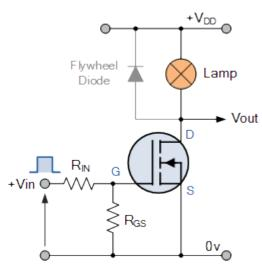
In this circuit arrangement an Enhancement-mode N-channel MOSFET is being used to switch a simple lamp "ON" and "OFF" (could also be an LED).
