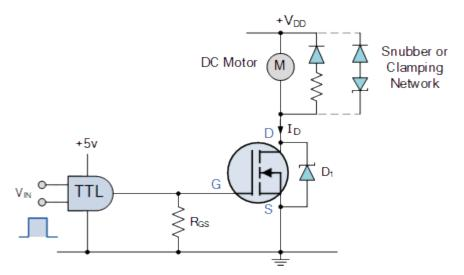
As the motor load is inductive, a simple flywheel diode is connected across the inductive load to dissipate any back emf generated by the motor when the MOSFET turns it "OFF". A clamping network formed by a zener diode in series with the diode can also be used to allow for faster switching and better control of the peak reverse voltage and drop-out time.
