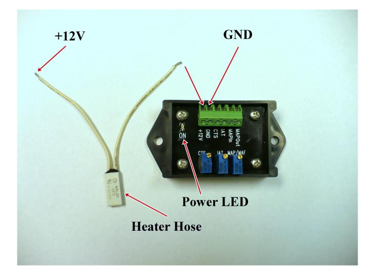
With the new Tstat switching device, you will need to solder on lengths of wire to the Tstat stub wires in sufficient length to reach your 12 v ignition switched power source and to reach the 12v input of your Tuning 101 Automated AFR Control Center. Refer to above photo. Connect your terminal marked GND to either the negative terminal of the battery or a GOOD clean chassis ground.
